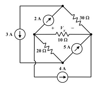
Use the superposition method to determine the value of  $V_{x}$ .
